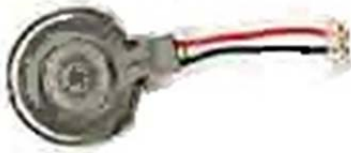
Fig. 5: Snapshot of a vibration motor
