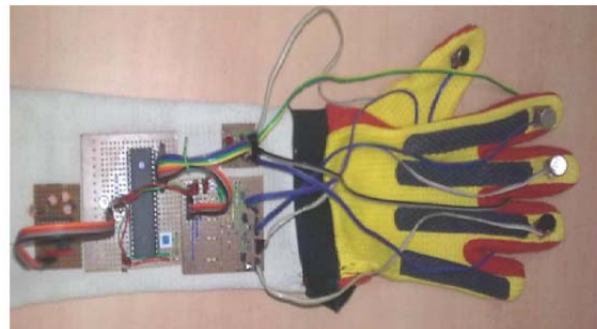
Fig. 7: Snapshot of the work with the vibration motor circuit at gloves
